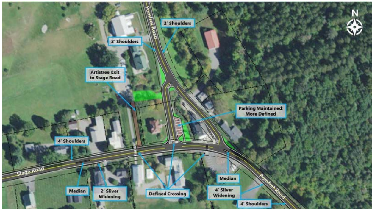
Figure 17: Alternative 1 Intersection Improvements
