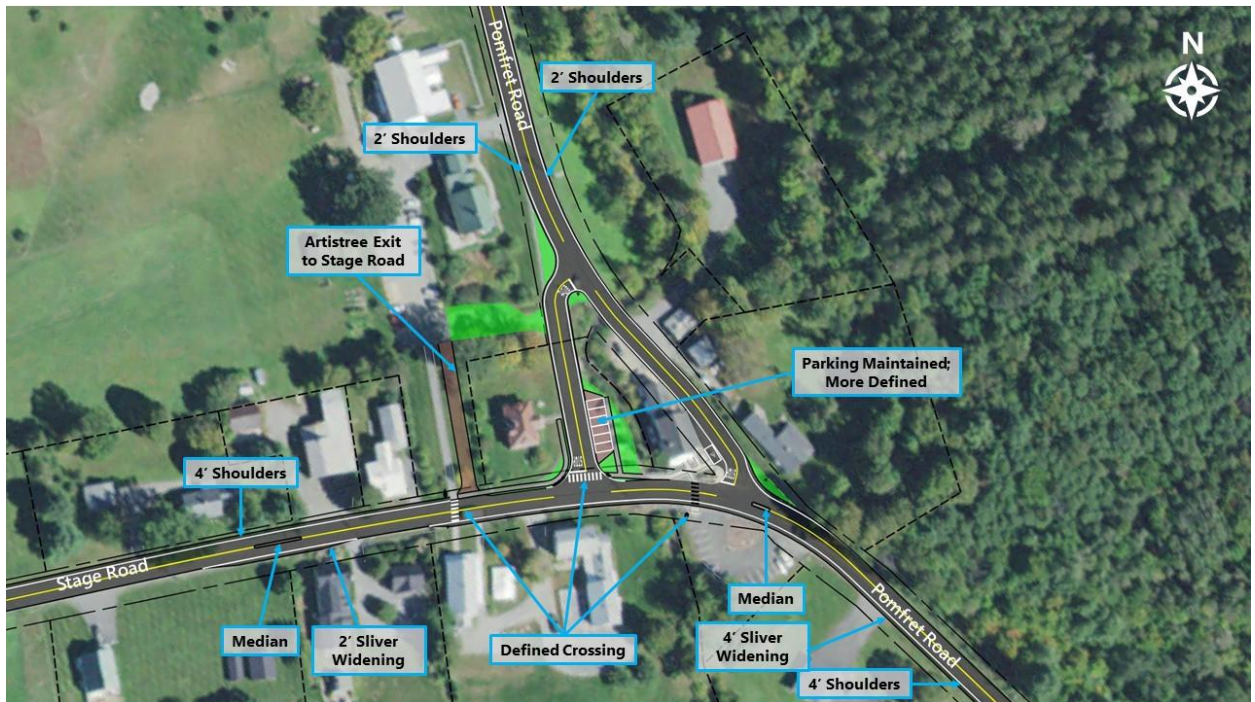
Figure 17: Alternative 1 Intersection Improvements
