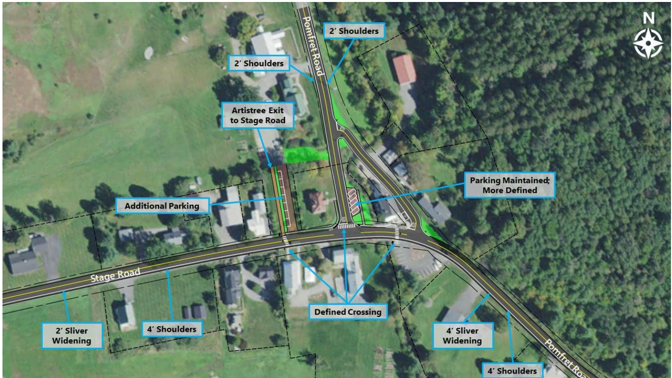
Figure 20: Alternative 2 Intersection Improvements
